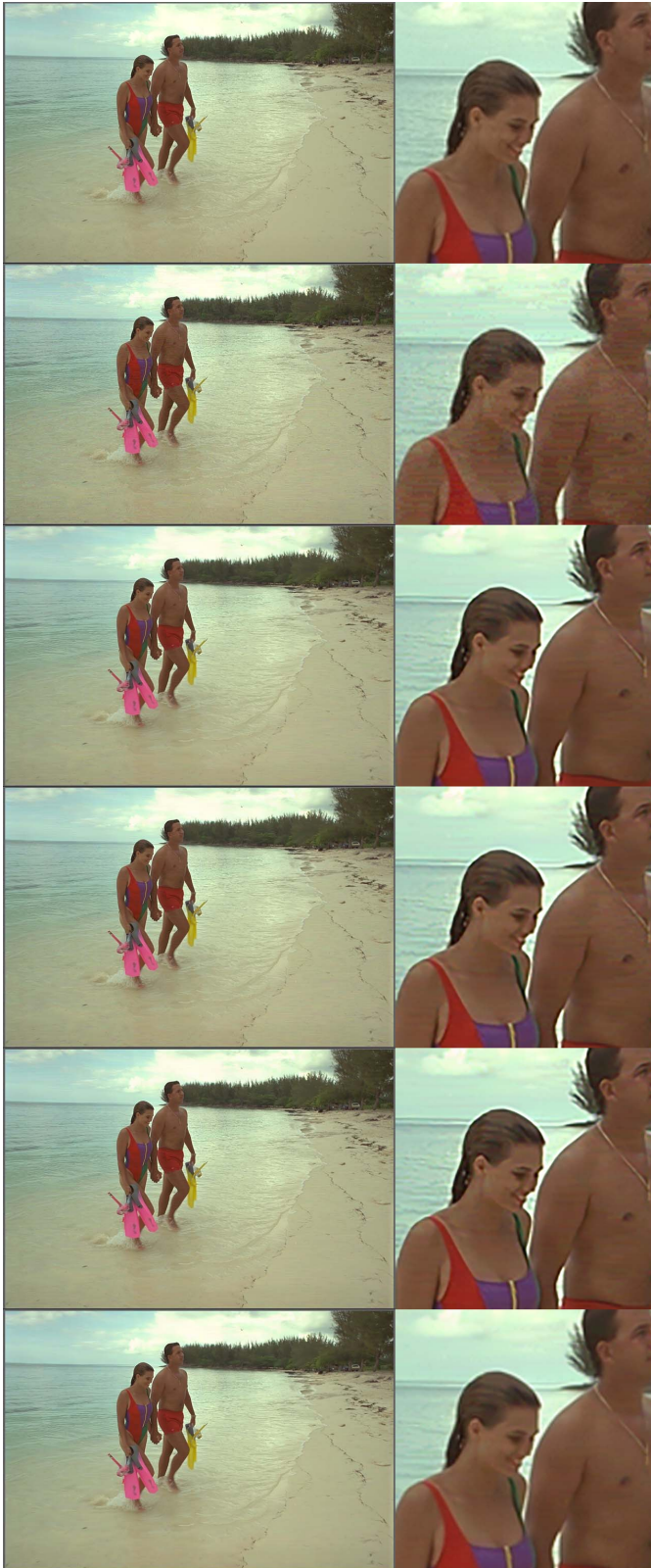
Fig. 17. Visual comparisons in colorful image ( kodim12 in Kodak PhotoCD dataset, \tau = 10 ). From top to bottom are the original image, NL-CALIC-coded image (PSNR/SSIM), GhostNet-decoded image (36.77/0.9772), PAN-decoded image (36.50/0.9758), MIRNet-decoded image (36.92/0.9780) and WRSD-decoded image (37.64/0.9816), respectively.
